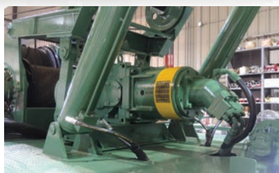
An optional integrated spudder mounted forward of the drawworks offers a max output speed of 31 rpms and a max operating torque of 13,750 ft. lbs.
