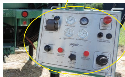
The operators console is located at the rear of the rig and conveniently located for excellent visibility and operator comfort. The operator's console includes drum, winch, mast, cathead & catworks controls including an emergency shutdown.
