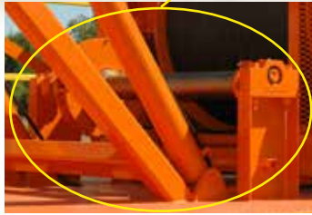
Deck mounted fleetings compensator, mounted behind drawworks. The compensator assists in spooling during "cross-county" on other non-conventional swabbing operations.
