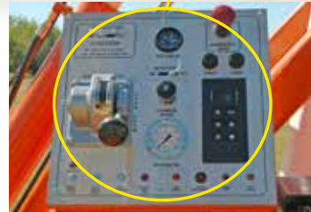
Drum controls including the brake lever, clutch control, gear selector, engine throttle and emergency shutdown are located on the operators console at the rear of the rig. Conveniently located for excellent visibility and operator comfort.
