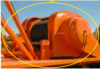
Drawworks is a single 42x8 band brake style drum. Design utilizes a forward mounted gearbox, chain drive and 24" single plate clutch to power the drum.
